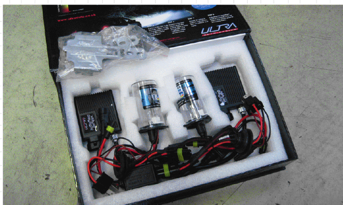
1) There are a wealth of xenon conversion kits available on the aftermarket scene. For the purposes of this guide we bagged a product manufactured by Ultra called the Virtual Daylight kit that retails for around £100 from most good stockists. Above right: HID bulbs are often visibly longer than the regular halogen bulbs
