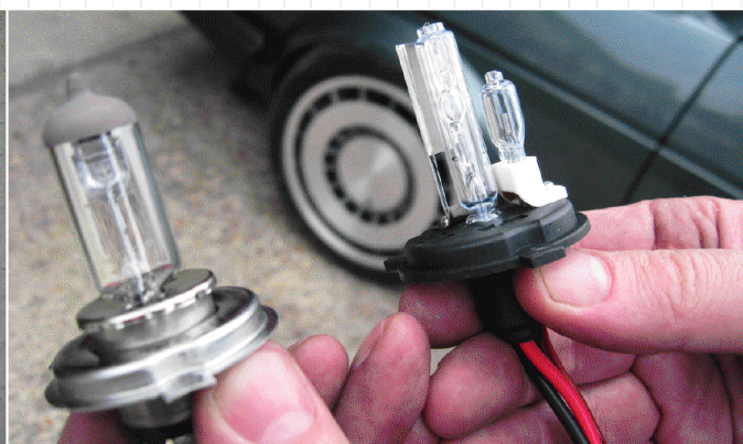
1) There are a wealth of xenon conversion kits available on the aftermarket scene. For the purposes of this guide we bagged a product manufactured by Ultra called the Virtual Daylight kit that retails for around £100 from most good stockists. Above right: HID bulbs are often visibly longer than the regular halogen bulbs
