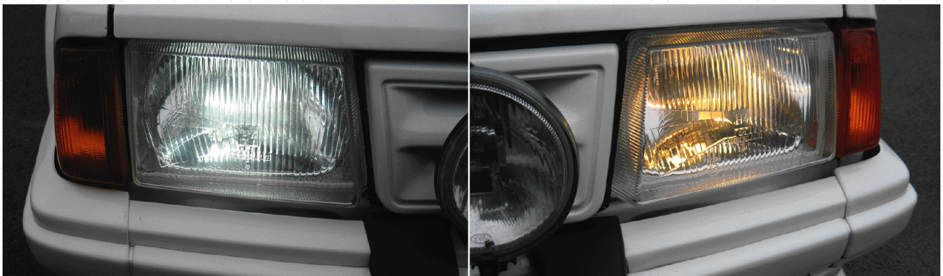
Above: Here you can easily spot the difference between the old lighting and new. The higher the Kelvin rating of the bulb the more purple the light will look. OEM kits run to around 4000K, most aftermarket kits are rated at 6000K (as seen here) or 9000K, some are more still but all have an impact on the kind of light you're generating
