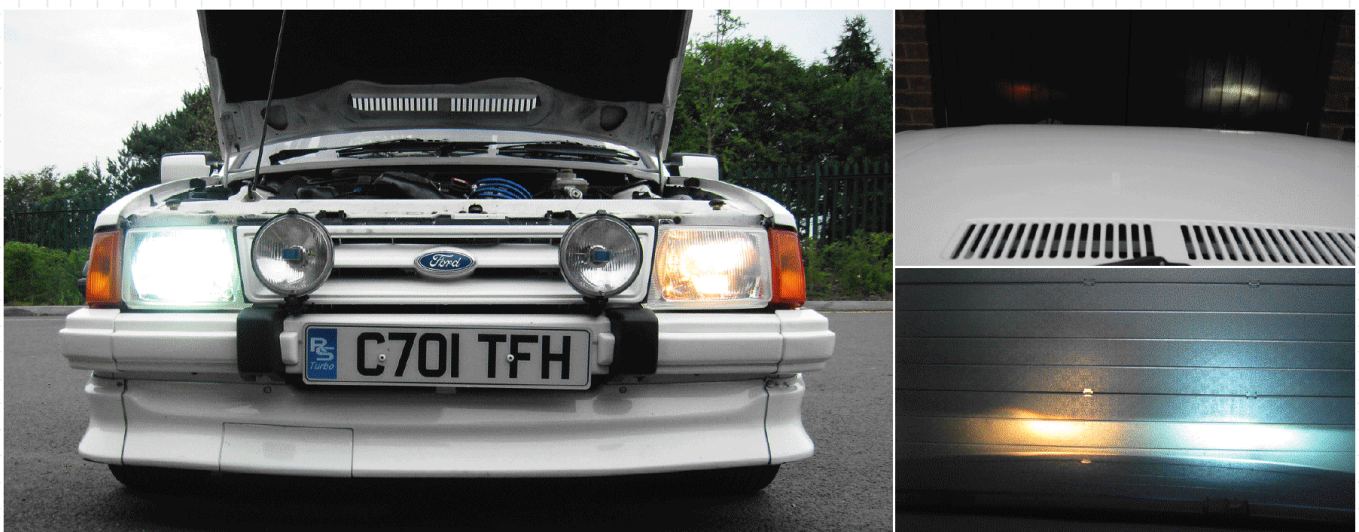
We parked the car up against the workshop roller door to get a good idea of alignment and beam pattern. This is one of the most important parts of the conversion, a badly aligned bulb will cost you at the MoT station...
